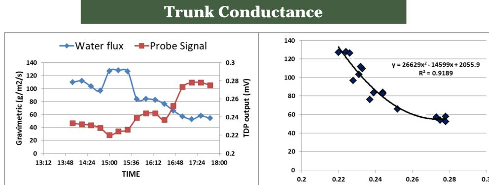
The pressure head was adjusted resulting in variable flux, which is noticeable as stepwise changes both in gravimetric (measured flux) and mV (TDP) readings over time. These steps created averages which were then used to determine the points on the graph below.
