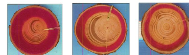
TDP error was evident in cross-sectional cuts, showing the probes exceeding the sap wood area on several samples.
