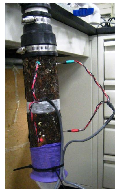
TDPs inserted in a sample with variable water pressure head.
