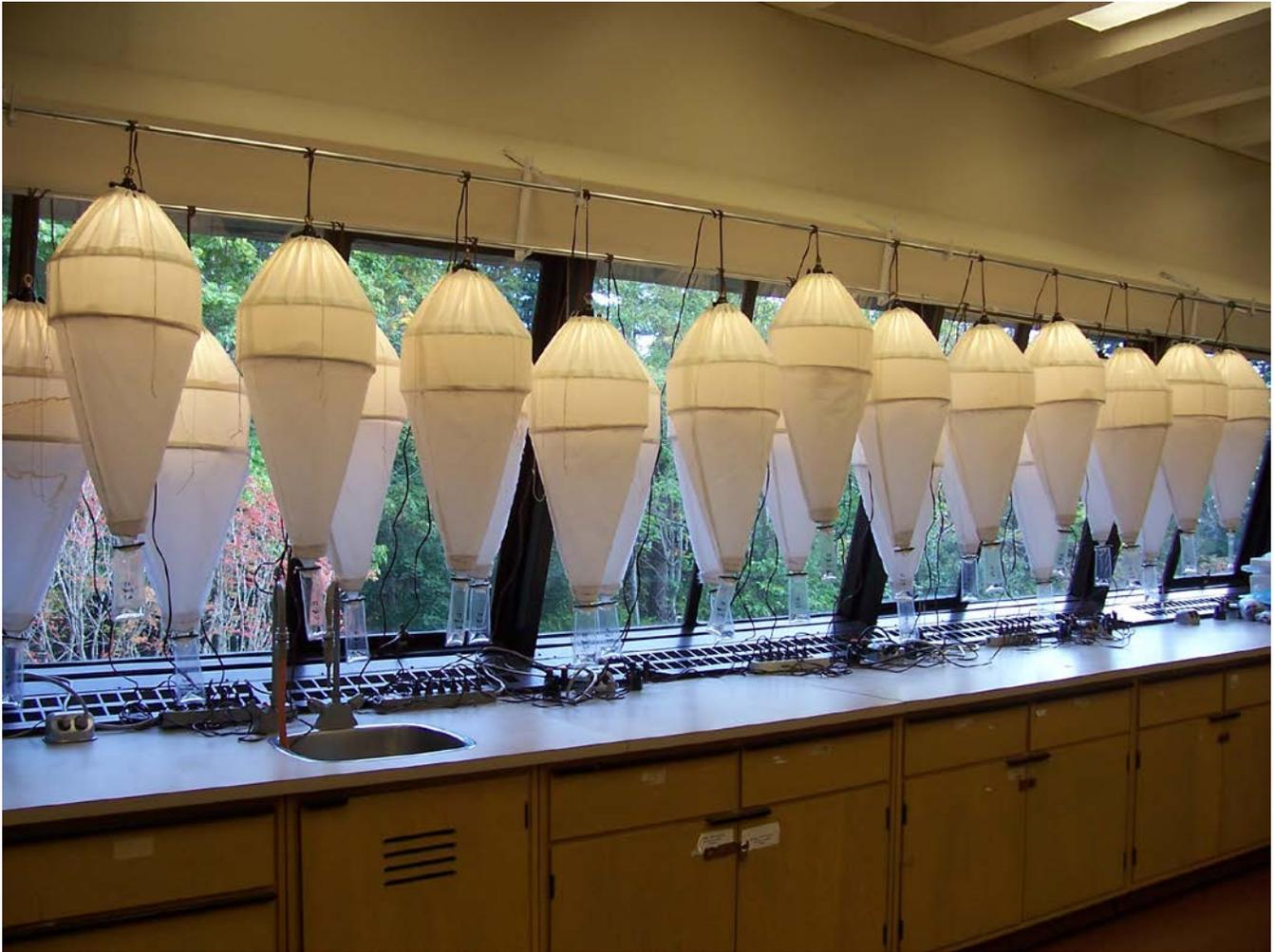
Portable soil fauna extractors called Berlese funnels work by creating a temperature / moisture gradient on soil samples; fauna actively move lower in the soil profile to be collected in 75% Ethanol at the bottom of the funnel. Temperature / moisture gradients are created using 40w incandescent lightbulbs.
