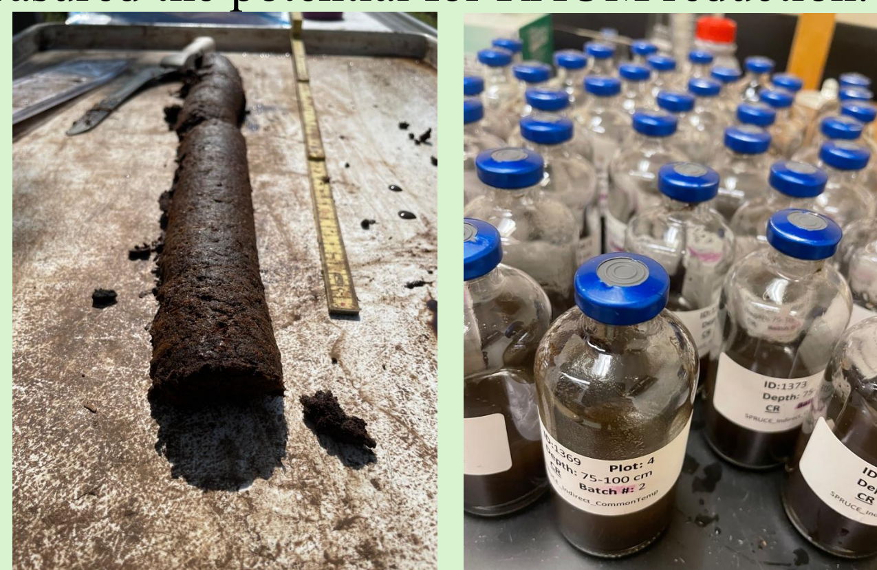
Fig. 5. Peat was collected from each experimental plot using a Russian corer (left) and placed in bottles to create peat slurries (right).
