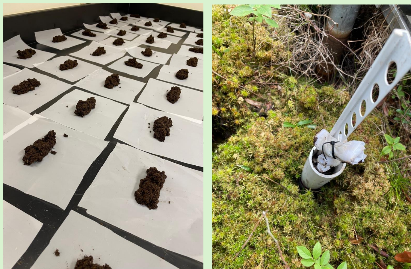
Fig. 3. Packets of peat (left) assembled and attached to a rod along specified depth increments and placed inside a peeper (right) within each experimental plot.
