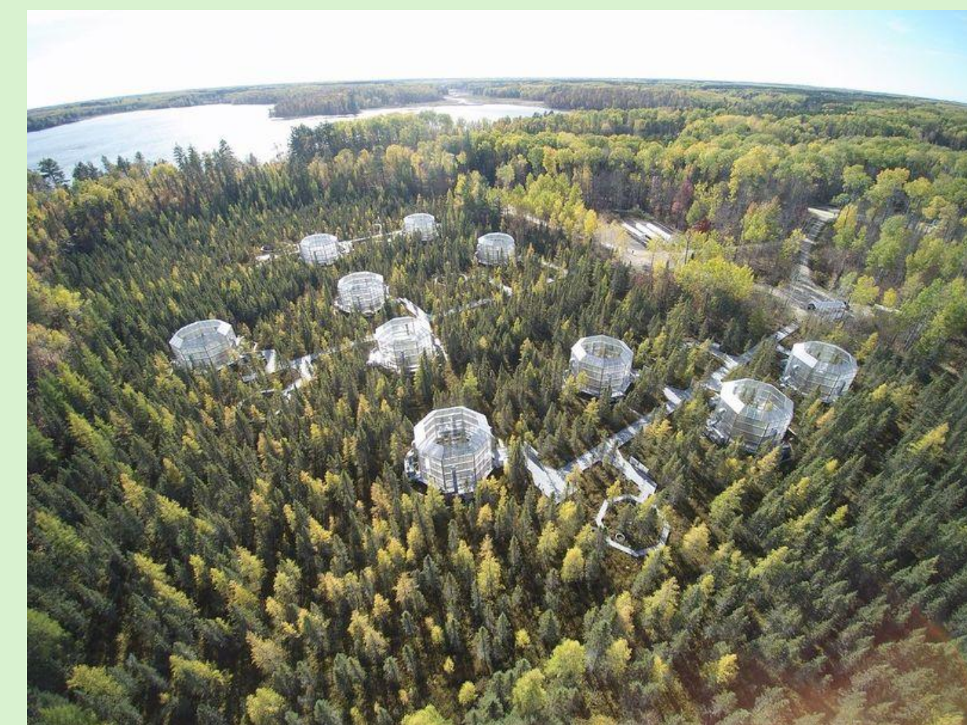
Fig. 2. The SPRUCE site has been exposing a peatland to whole-ecosystem warming (WEW) and elevated atmospheric CO 2 (eCO 2 ) since 2014.
